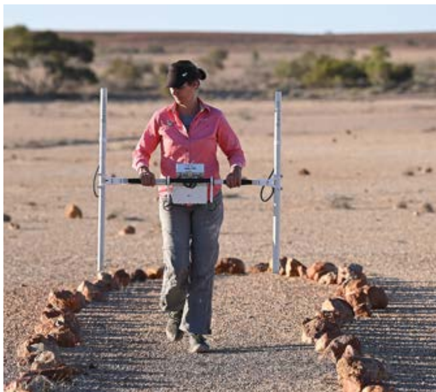
The Bartington Instruments Fluxgate gradiometer used to map Mithaka stone arrangement, 2021. Photo: L. Mechielsen
